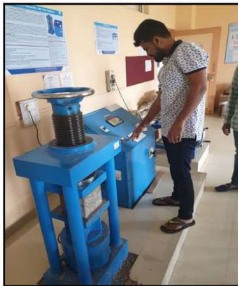
Figure 2. Performance on Compression Test Machine
